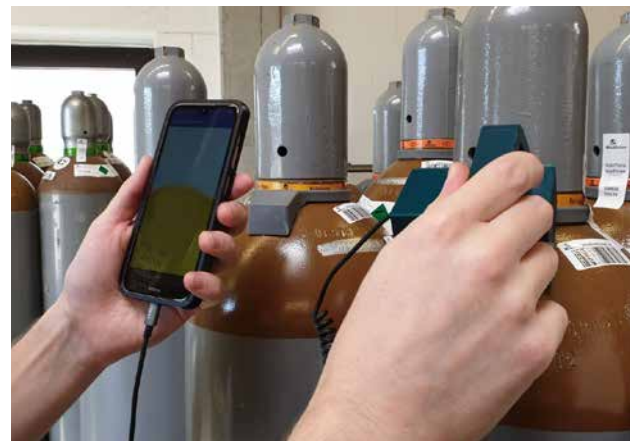
The Smart Track project is developing RFID chips and scanners that can be used to automatically track and monitor gas cylinders.
