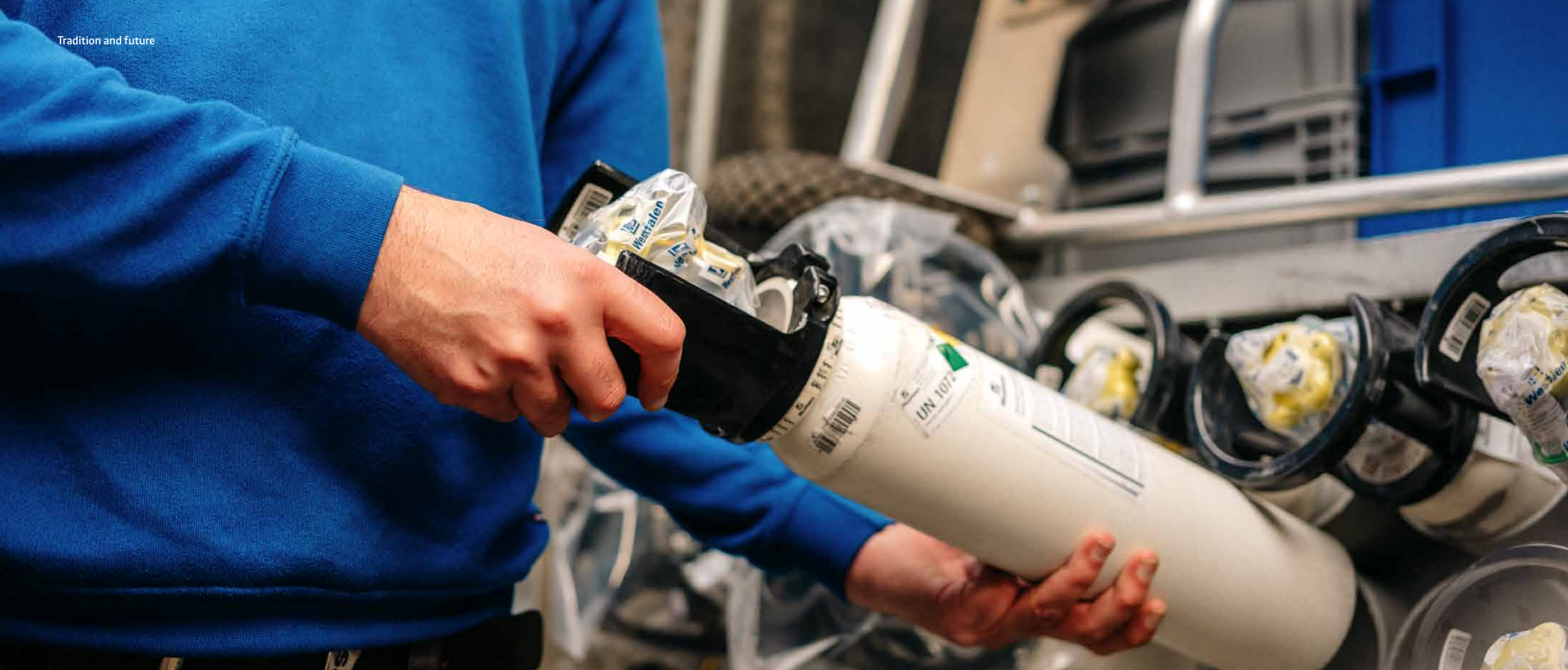
Cylinders with medical oxygen for the supply of patients in the homecare sector.
